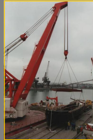
Using a 400 tonne capacity "Mega Lift" system in order to undertake the removal of three 70 tonne furnaces prior to transportation to Liverpool for export.
